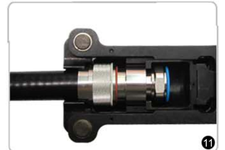
Put the connector into the compressing frame and make sure connector being sitted steadily.
