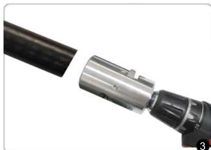
Insert the cable into the trimming tool. Select the low speed on the drill or 400~600 RPM on a variable speed drill. Trim the cable.
